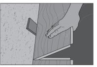
planks are perfectly aligned. Install remaining full planks in the first row.
