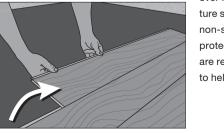
slightly knocking just above the joint Fold up and release the whole long side. Disassemble the panels by sliding horizontally. (Do not fold up!)
